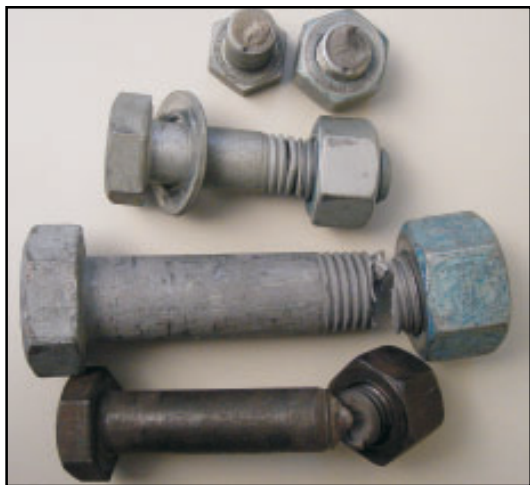
Figure 1: Heavy Hex Bolt Breakage
