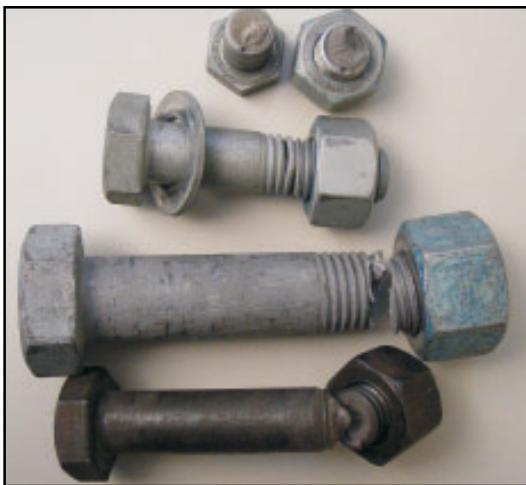
Figure 1: Heavy Hex Bolt Breakage
