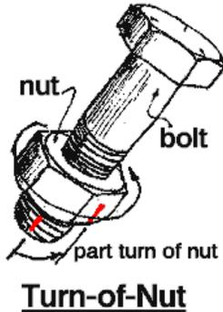
Note: As with every bolt pretensioning method, Turn-of-Nut may only be performed after all steel plies in a connection have been drawn into firm contact, i.e. snug-tightened. Failure to do so will result in inadequate bolt pretension and loose connections. Also, The Pre-installation Verification fastener testing must be conducted per applicable AISC/RCSC sections with the caveat that Turn-of-Nut verification may not be verified by Direct Tension Indicator verification (AISC/RCSC 16.2-59).
