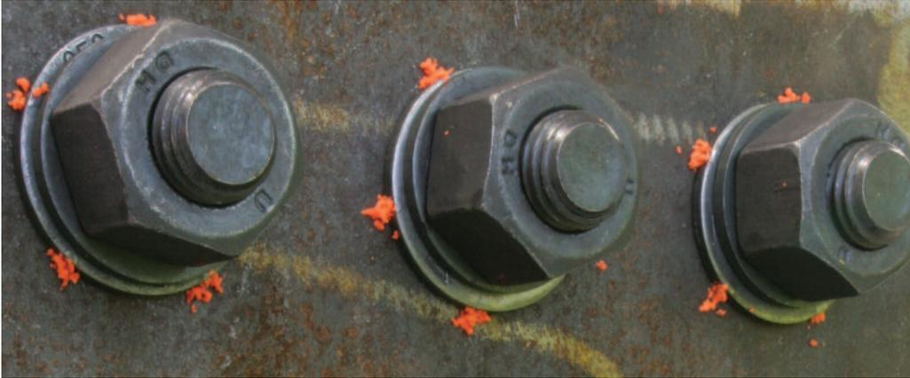
Squirter®DTIs are DTIs with a flexible silicone embedded in the depressions under the bumps. **To use them, simply ...** Tighten the bolt until the calibrated amount\* of orange silicone appears from under the DTI's squirt locations, then stop tightening. **That's all there is to it.**
