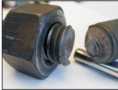
Figure 4: How to identify a torsional failure; conical shape and a spiraling to the grain of the bolt.
