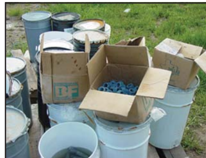
Figure 2: Kegs left unprotected in the weather will increase the torque needed as well. Did you notice the water in the keg?
