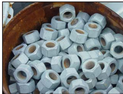
Figure 1: An open keg of galvanized nuts without any visible dye lubricant with rusty threads. This will definitely increase the turning resistance making the bolt assemblies more difficult to tension.
