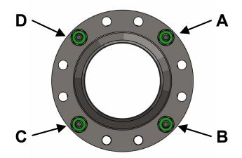
Insert **four** fit-up studs; one in each quadrant.
