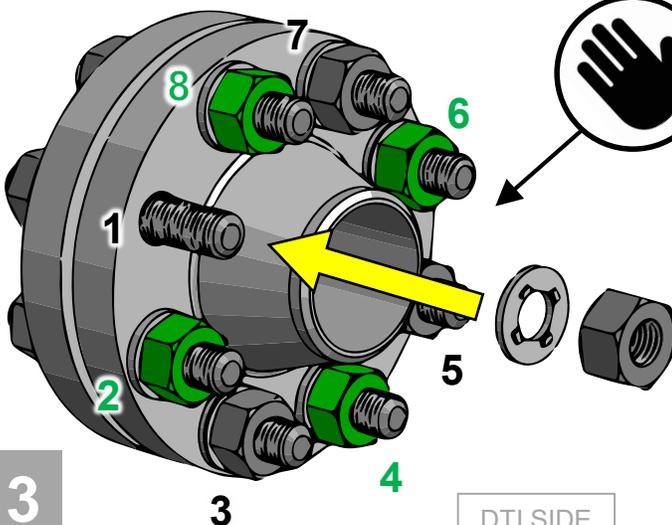
Insert and **hand tighten** the remaining hardware, now including DTIs.
