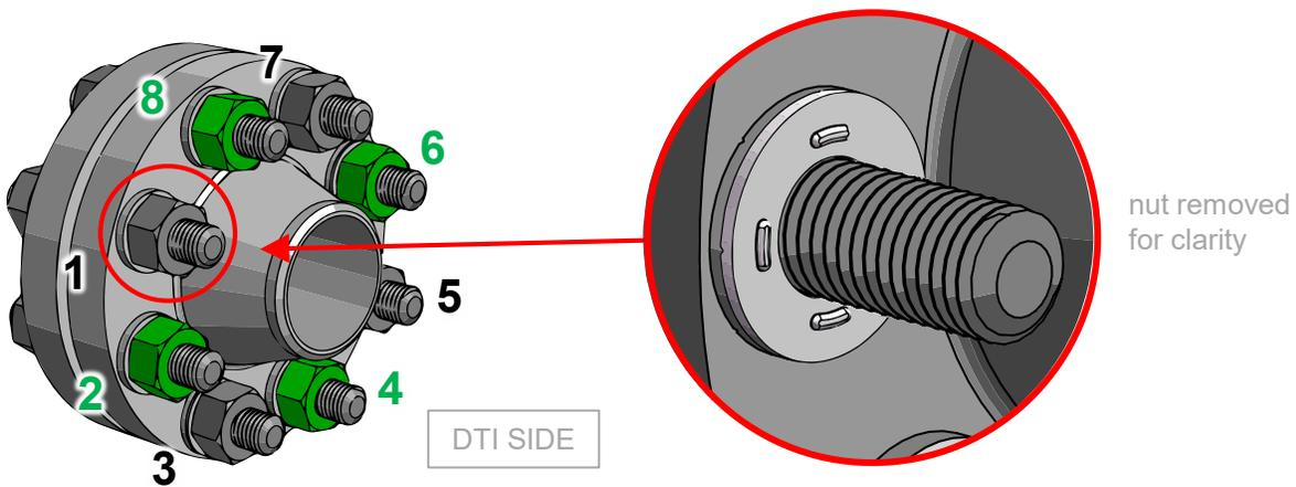
**4** Confirm the DuraSquirt DTIs were installed correctly and the fit-up ones are available, which will get installed in step 6.
