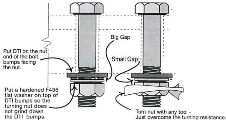
DTI's are individual bolt load cells, which measure pretension developed during tightening, regardless of torque resistance of the bolt. By far the simplest method, a DTI is put on one end of a bolt and tightened until the bumps are compressed enough so that a feeler gage cannot be inserted all around, or when the Squirter® DTI has deployed silicone properly. DTI's are completely independent of torque resistance of the bolt assembly, and because the
