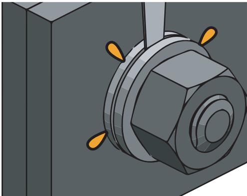
Confirm the gap is smaller than the calibrated gap provided by Applied Bolting Technology.
