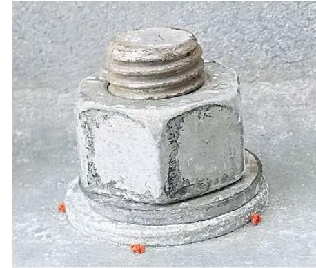
DuraSquirt® DTIs may be installed and inspected visually, regardless of environment or elapsed time between initial installation and inspection.
