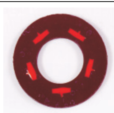
1. Loctite® silicone in DTI cavities
