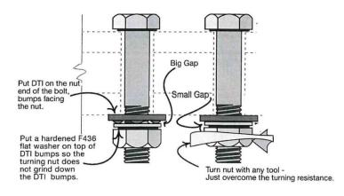
DTI's are individual bolt load cells, which measure pretension developed during tightening, regardless of torque resistance of the bolt. By far the simplest method, a DTI is put on one end of a bolt and tightened until the bumps are compressed enough so that a feeler gage cannot be inserted all around, or when the Squirter<sup>®</sup> DTI has deployed silicone properly. DTI's are completely independent of torque resistance of the bolt assembly, and because the
