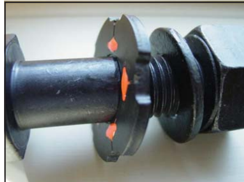
Figure 7: Iceland Fjardaal Project Xylan Coated Bolt/DTI
