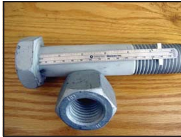
Figure2: Dacromet Coating Boeing Bolt
